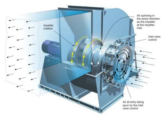
With radial vane control the guide vanes are positioned directly in front of the impeller eye and therefore produce a more uniform and efficient spin. Inlet louvre dampers are fitted into an inlet box. The style of vane control that should be used depends on the conditions that the fan will be operating as well as restrictions on space.
