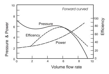
The forward curved impeller produces very high pressures compared to other centrifugal fan types with the same impeller diameter and running speed. Only the radial style of impeller is capable of producing a higher peak pressure. The high tip velocities ensure that the volume flowrate for this type of fan are very large.
