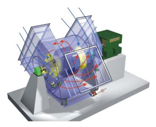
The blue arrows show the flow through the inlet boxes, whilst the red arrows indicate the flow through the casing.
