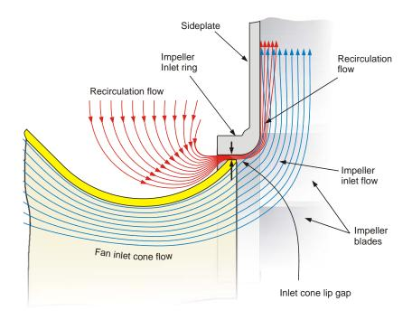
As the air flows through the gap between the impeller and inlet cone, it will tend to stick to the sideplate. The airflow from the inlet cone will then tend to flow toward the air at the impeller sideplate and bend through 90° to fill the impeller.
