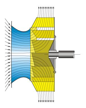
For an open inlet centrifugal fan, the inlet cone is the first part of the fan that the airflow comes into contact with. It is vitally important that the air is guided into the impeller inlet, otherwise the impeller will not operate efficiently and the performance will be greatly reduced.
