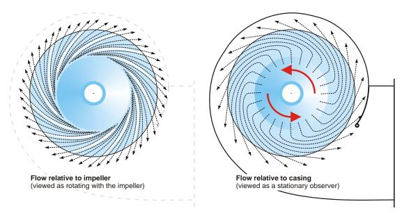
W is the relative air velocity – this is the velocity of the flow relative to the impeller. The relative velocity at the impeller outlet is in the same direction as the blade tips.
