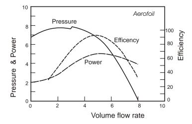
For the same diameter and running speed this style of impeller produces significantly lower pressures than the plate bladed impeller. However this impeller style can offer large volume flowrates in the operating range.
