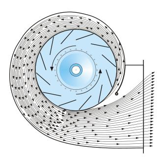
The purpose of the casing is not only to collect the air leaving the impeller and to point it in a useful direction, but also to transfer a significant proportion of the dynamic pressure from the air, which is leaving the impeller, into more useful static pressure.
