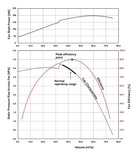
The performance of a centrifugal fan may be described in terms of pressure and volume flowrate. A pressure-volume curve is used to display the relationship between the pressure and volume flowrate for a particular fan, this curve is known as the fan characteristic. A typical characteristic is shown above.
