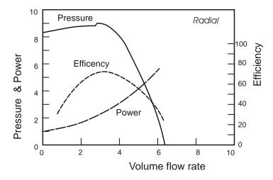
This type of impeller develops the highest total pressure of any of the centrifugal impeller types, for the same impeller diameter and running speed. This is due to the high tip velocities that are produced. However the inefficiencies in the flow mean that the attainable flowrates are low and the pressure drops off
