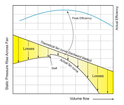
The theoretical characteristic for a fan is a straight-line, however rotational losses, friction and incidence will reduce the actual pressure that is attainable. Incidence is the difference between the fluid and blade angles at the impeller inlet
