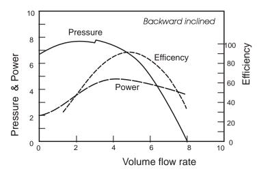
This impeller style develops a lower peak pressure than the radial impeller but offers a significantly higher volume flowrate for the same impeller diameter and running speed. The stall characteristic is similar to that for a radial bladed impeller.
